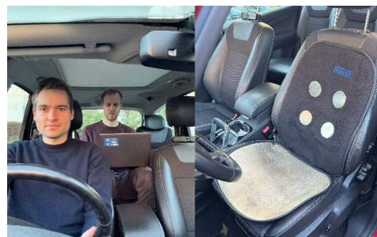
Fig. 7: Unobtrusive measurement of cardiovascular parameters on the driver's seat. Left: Our colleague, Daniel Blase, sitting on the integrated sensor system, and Markus Lüken in the back seat recording cardiac signals. Right: Integrated sensing system on the driver's seat. Fusion of Electrical Impedance Tomography & Ultrasound Tomography
