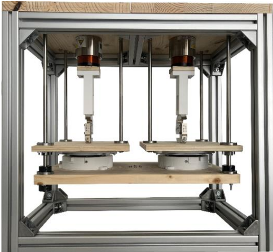
Fig. 4: Scheme of the cECG test bench. Using two voice coil actuators, the contact pressure of both elec-trode-skin interfaces can be controlled individually. This allows testing with impedance mismatches between the electrodes as well as the modulation of dynamic contact pressures, as induced by cardio-mechanical activity.
